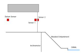
There is a question mark over the cause of movement to this two storey structure which has been built very close to a steep slope in the Mercia Mudstone.
